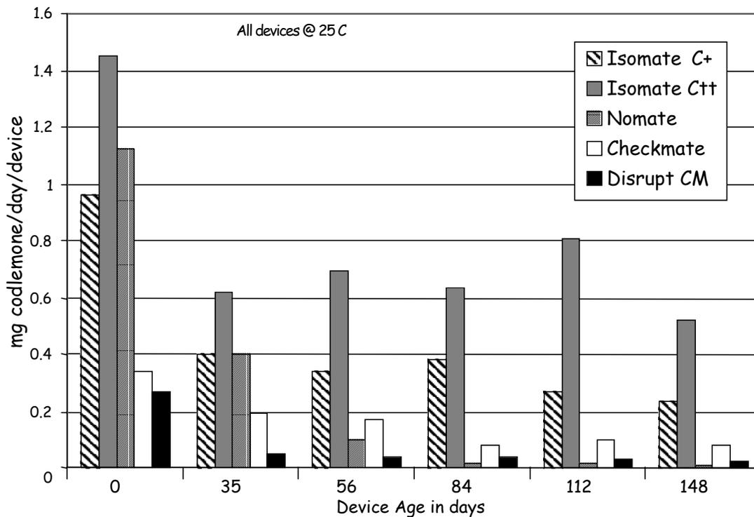
The VTS provides a relative comparison of the release rate of codling moth pheromone from dispensers of different ages in a dynamic environment. The one main concern we have about the
