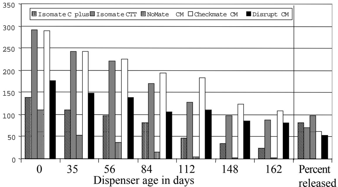
The desired release characteristic of a pheromone dispenser is termed a “zero order” release. This is where a constant release rate of pheromone would occur over time until the dispenser is
